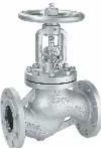
Item 346 flow valve, traditional type PN 40 / A 150 - 300 Carbon steel 1.0619 body Flanged with bellows stainless steelstem bellows and sealing seats press Max 40 bar Temp Max + 400° C
