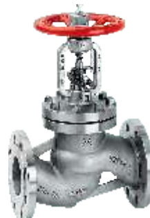
Item 347 flow valve with bellows PN 40 / A 150 - 300 Stainless steel GX5CrNiMo 19-11-2 body Flanged with bellows With stainless steel stem bellows and sealing seats press Max 40 bar Temp Max + 400° C
